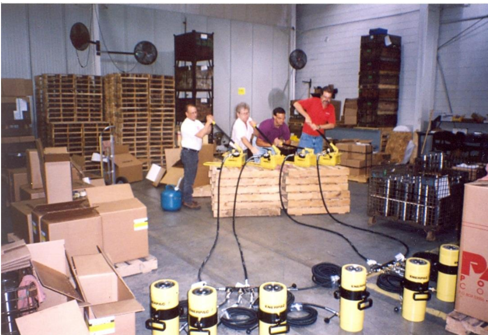
Load Testing Two 400 Ton Jacking Systems
